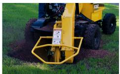
AUTOSWEEP® SYSTEM. Optional. The AutoSweep function monitors engine speed and automatically adjusts cutter wheel sweep rate, and is designed to reduce engine, drivetrain and structural stress.
