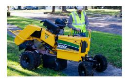
TWO-SPEED GROUND DRIVE. The operator may choose to operate in a high-range or low-range ground speed setting of 0-133 ft/min (0-40.5 m/min) to quickly move the machine or choose a slower speed when near the stump by utilizing a low-range setting of 0-66 ft/min (0-20.1 m/min).
