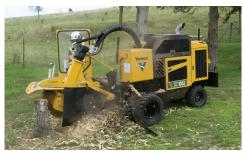
4-BAR LINKAGE. Maximize cutting width through a unique 4-bar linkage that moves the cutter wheel away from the machine as the boom drops. This helps the cutter wheel grind the stump at all maximum dimensions.
