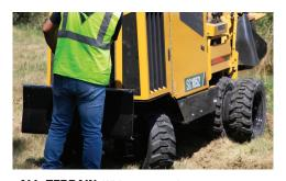
ALL-TERRAIN. With power and torque transferred to each of the four wheels, the SC1052 is able to traverse difficult and uneven ground conditions, with minimal ground disturbance. With the differential locks disengaged, maneuverability is enhanced. In difficult ground conditions, the operator can engage the differential locks to maintain pulling power during uneven wheel traction conditions.
