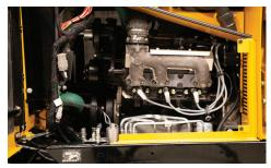
MORE POWER. The 115-hp (86-kW) gas engine provides high productivity and speed, resulting in maximum cutting power and minimal maintenance needs, to help you complete more jobs in a day.
