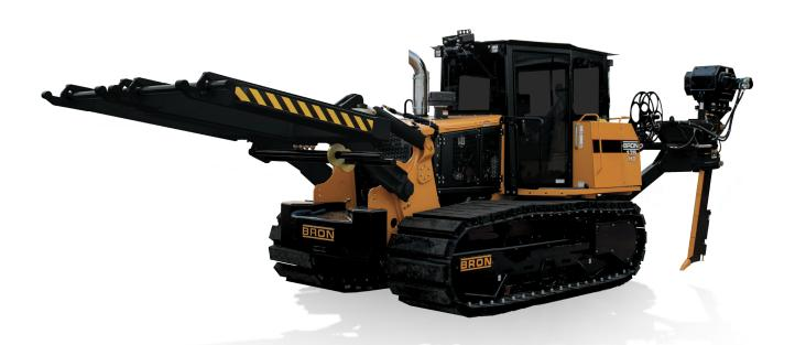
The BRON 175HD is a compact Utility Tractor used for gas and utility installations. Engineered for power and performance, the BRON 175HD is designed to allow contractors to work on any terrain, manoeuvre in tight areas, and perform effectively in all soil conditions. The BRON 175HD comes with variable vibration for optimal performance in tough ground conditions along with an 8,000 lb. capacity reel carrier.
