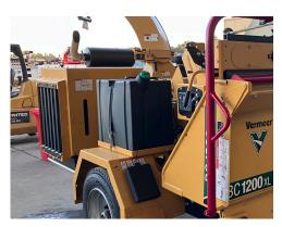
**EASY CONTROL ACCESS.** The operator's control panel and combination clutch/throttle control handle are conveniently located towards the rear of the machine.
