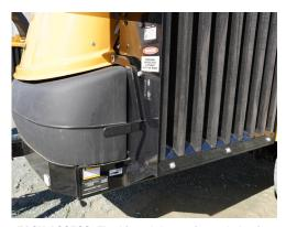
**EASY ACCESS.** The hinged thermoformed plastic engine enclosure design helps with easy access to maintenance points and limited noise.
