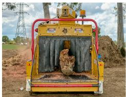
**CHIPPING PRODUCTIVITY.** The SmartFeed system monitors engine rpm and automatically stops and reverses the feed rollers to enhance production. This system also senses feed roller jams.
