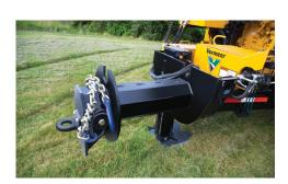
JOBSITE MOBILITY. The WC2300xL has a compact design and built-in skidder grab on the tongue, allowing it to be moved around on the jobsite by a skidder or excavator.
